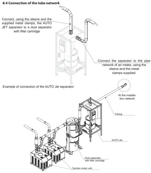
The sizing of the suction unit and of the suction lines leading to the Auto Jet Turbix must be made giving consideration to the number of simultaneous users and the type of material to be vacuumed.
