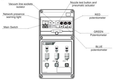
**Main switch:** magnetotherrmic switch for isolating and protecting the power supply line of the control panel.
