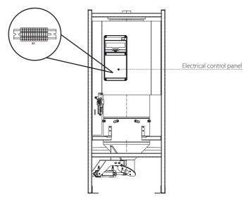
Open the front cover of the control panel to gain access to the terminal block for the electrical connections.
