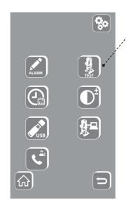
Press the button to access the following tests: AUTOCLEANER FUNCTIONALITY (optional) VACUUM SYSTEM FUNCTIONALITY VACUUM SOCKETS FUNCTIONALITY CAN BUS CONNECTION CHECK
