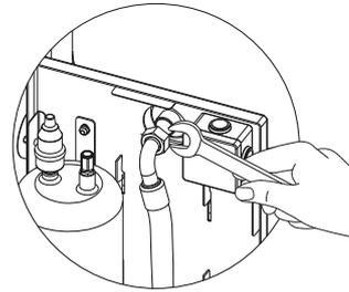
2 - Screw the connection (female) on the entrance (male) using the supplied gasket, keeping it tight.
