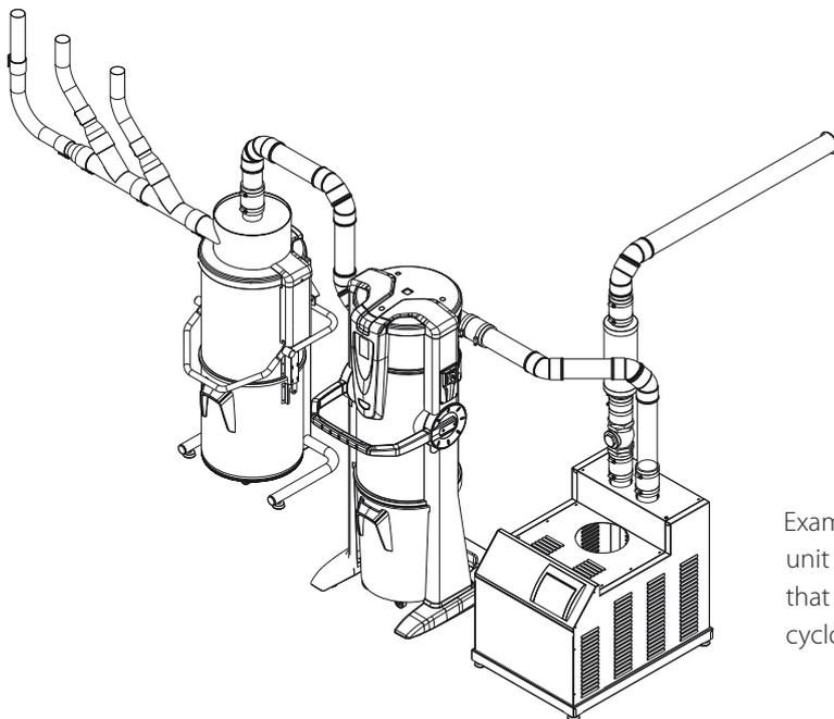
Example of central vacuum unit with three-line collector that converge in a Turbix cyclonic pre-separator
