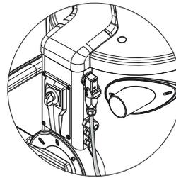
2 - Connect the plug on the Autocleaner and close the safety catch.
