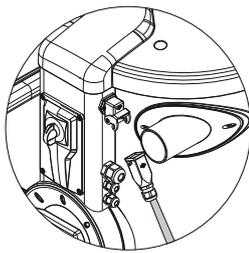
1 - Remove the connector cap on the vacuum unit.
