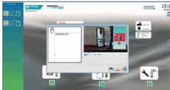
It is also possible to recall a video tutorial of the required maintenance, which was previously created and saved on the PC, in order to further simplify this operation.
