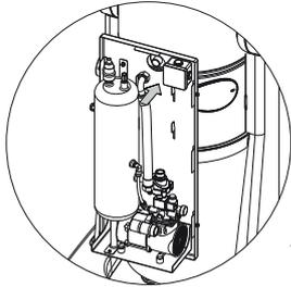
1 - After connecting the Autocleaner on the fixing bracket, position the compressed air hose fitting at the entrance at the rear on the back part of the vacuum unit.
